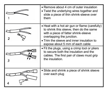
For connection to other hub dynamos see their instruction manual. If one contact of the dynamo is electrically connected to the frame (e.g. all models of Shimano), the wires are no longer interchangeable: the outer conductor of the coaxial cable (not insulated or covered with black shrink sleeve) must be connected to the ground, the transparent insulated interior wire must be connected to the phase contact of the dynamo.
